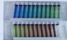
The recipe for reproducing the coloured liquids of the scale can be found in Marcel's thesis, *Posidon's Paintbox*, Chapter 4. 'Spectral analysis of the Forel-Ule Ocean colour comparator scale'. A mixture of three standard solutions is used to obtain the colour palette of the scale. The standard solutions are made with distilled water, ammonia, copper-sulphate, potassium-chromate and cobalt-sulphate.
